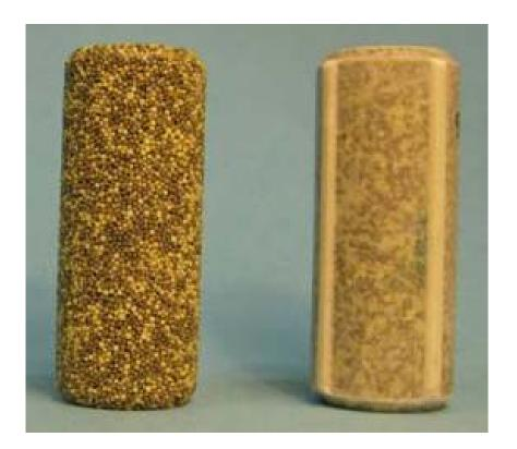
The propellant body is a cylindrical body made of glued double base ball powder (AkII stabilized) containing nitroglycerine.
