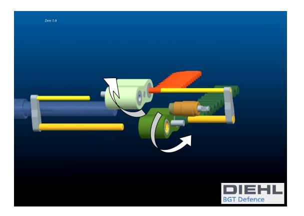
Loading the projectile (above) and the charge (below) simultaneously in the two different chambers.
