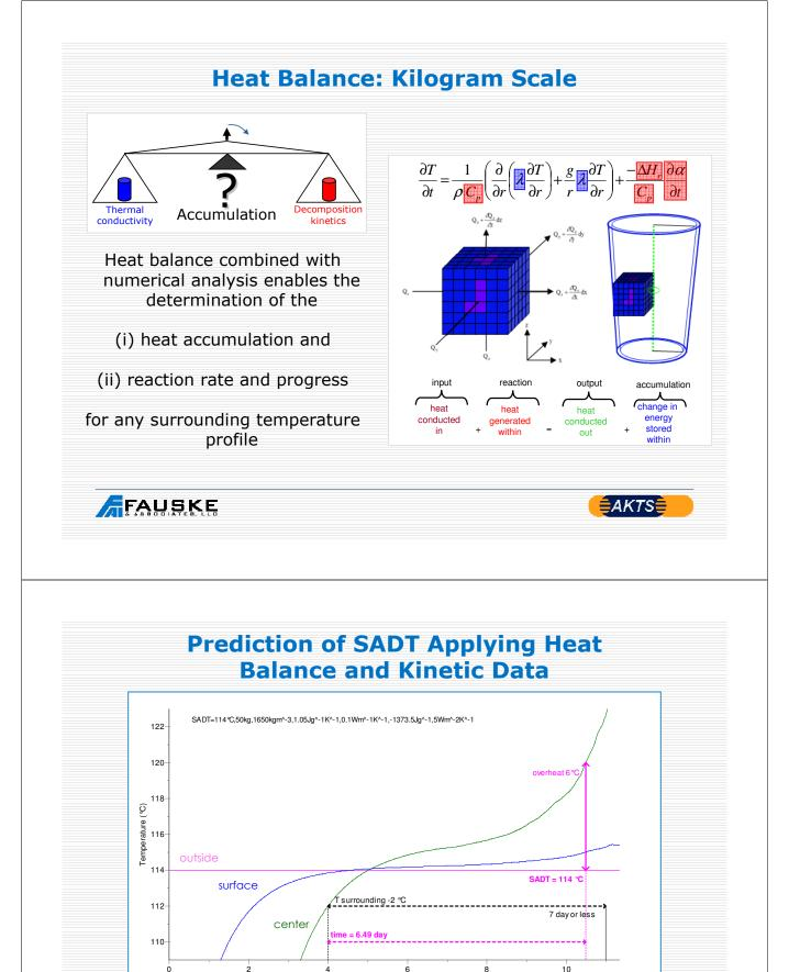
The SADT is 114℃. This temperature is the lowest environment temperature at which overheat in the middle of the specific packaging exceeds 6℃ (△T6) after a lapse of the period of seven days (168 hours) or less. This period is measured from the time when the packaging centre temperature reaches 2℃ below the surrounding temperature. This overheat of 6℃ occurs after about 6.5 days.
